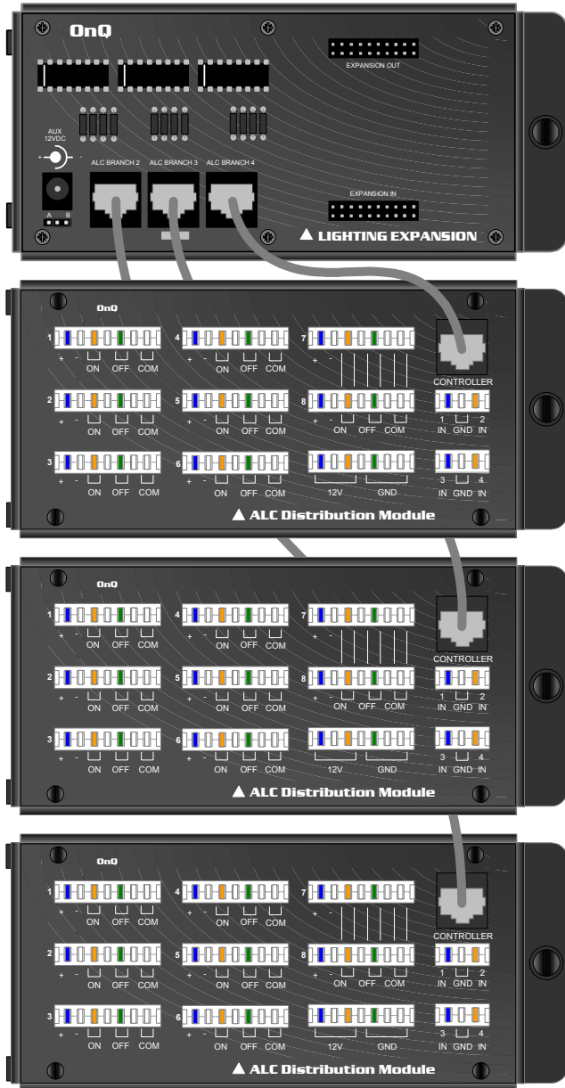
Figure 4. Lighting Expansion with Wiring Distribution
